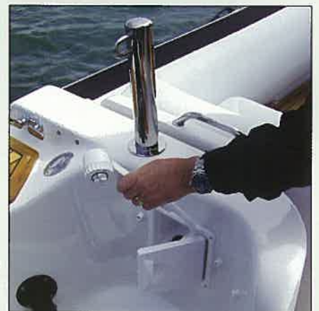
Fresh water washdown hose aft.
