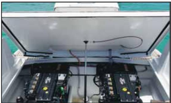
The aft third of the cockpit sole tilts electrically to access the engines.
